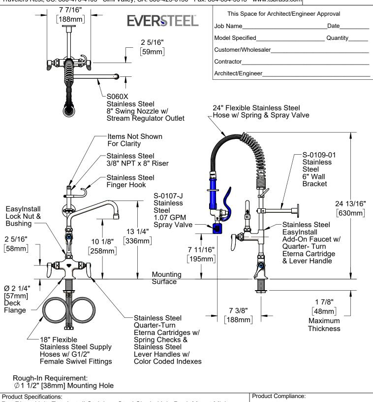
Pre-Rinse Unit: EasyInstall Stainless Steel Single Hole Deck Mount Mixing Faucet, SS Quarter-Turn Eterna Cartridges w/ Spring Checks, SS Lever Handles, SS Add-On Faucet, SS 8" Swing Nozzle, 24" Flexible Stainless Steel Hose, SS 1.07 GPM Spray Valve, SS 6" Wall Bracket & Flexible Stainless Steel Supply Hoses
