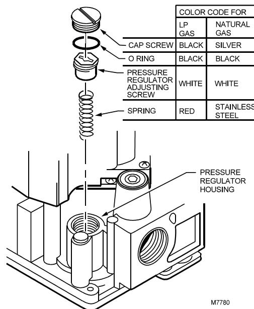
Installation of conversion kit in regulated gas control.
