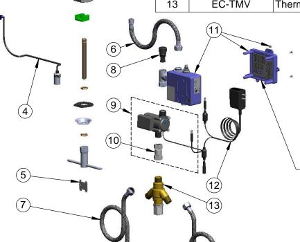
A Maximum of (8) ChekPoint Faucets can be Hardwire Connected and Powered by EC-HARDWIRE ChekPoint Hardwire AĆ Transformer. (Sold Separately)
