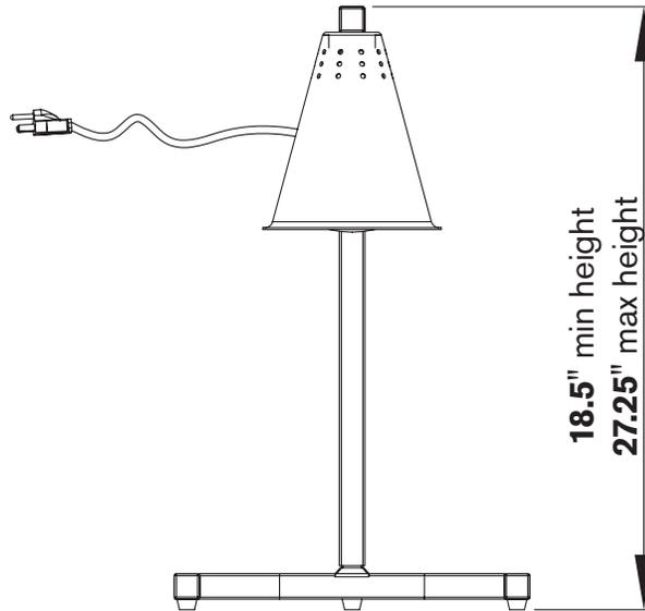
**Electric:** Attached 6-foot flexible, three-wire cord with ground plug (NEMA 5-15).
