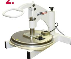
After setting time and desired thickness, swing upper platen over dough ball and pull down the handle until it locks into position. Using both hands, pull up the handle.
