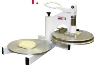
After allowing upper platen to reach desired temperature, place pre-portioned ball of dough in center of platen.
