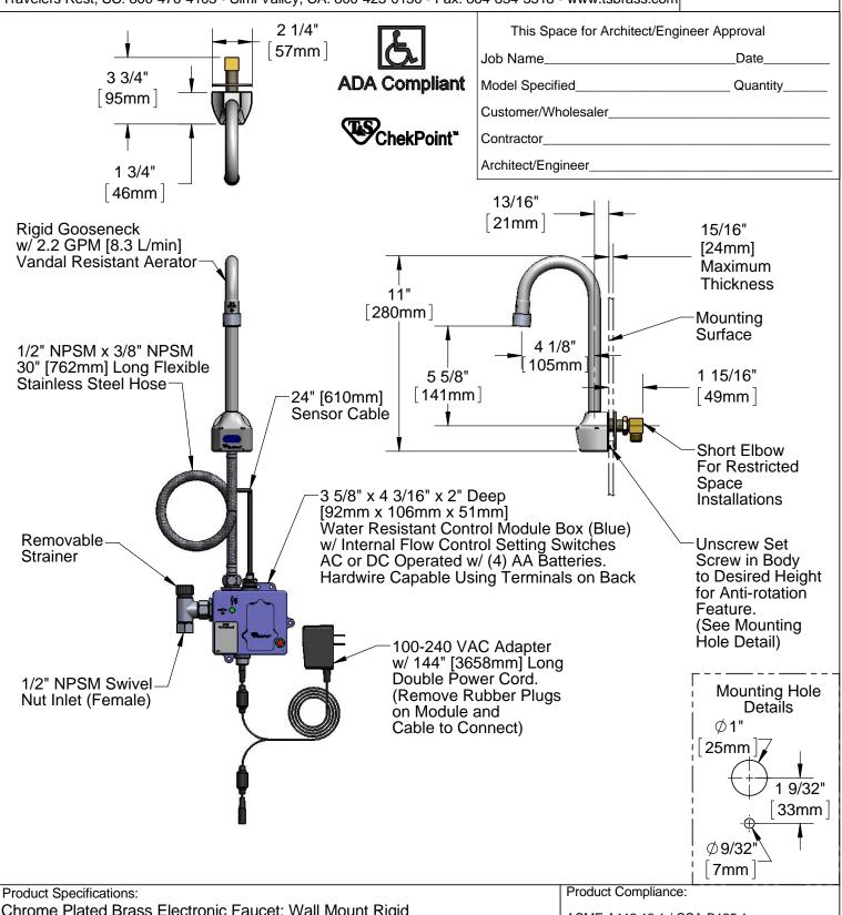
Chrome Plated Brass Electronic Faucet: Wall Mount Rigid Gooseneck w/ VR Aerator, AC/DC Control Module w/ Internal Flow Control Setting Switches
