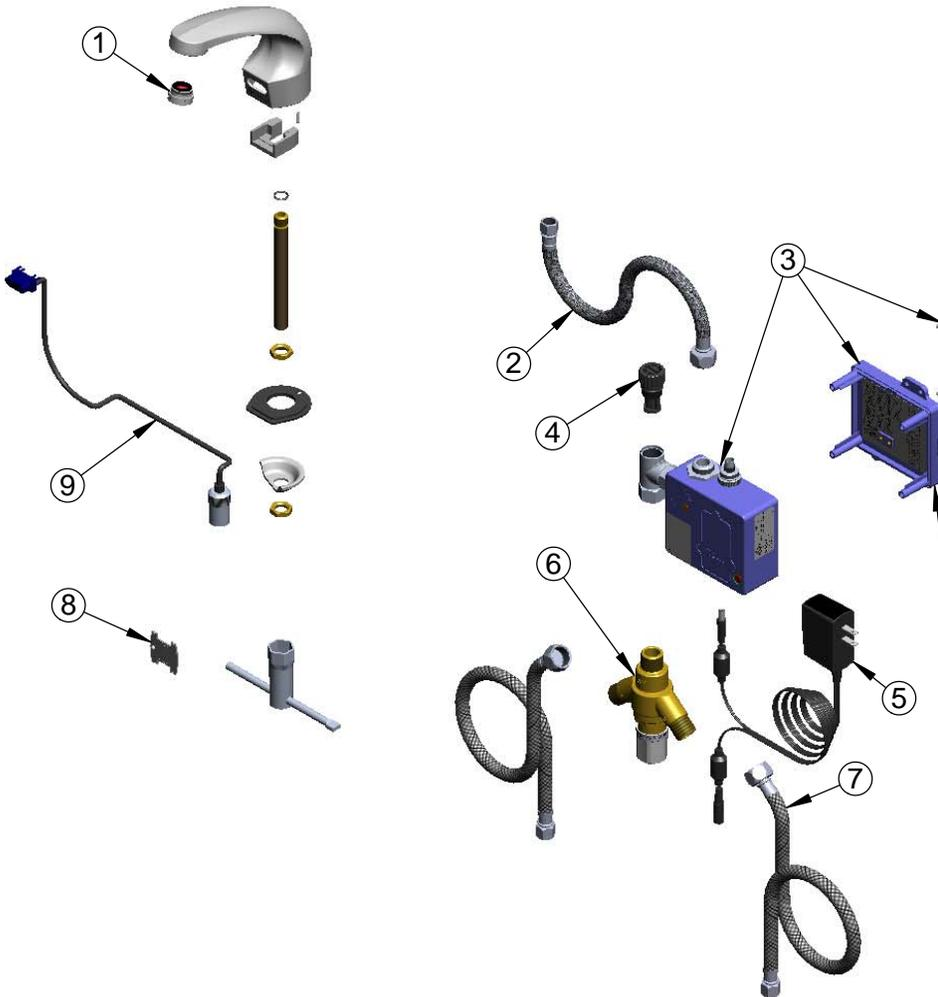
A Maximum of (8) ChekPoint Faucets can be Hardwire Connected and Powered by EC-HARDWIRE ChekPoint Hardwire AC Transformer. (Sold Separately)
