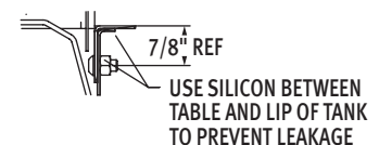
Sectional View Showing Table Connections
