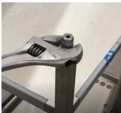
Figure 1 Use a wrench to remove UNISTAND foot
