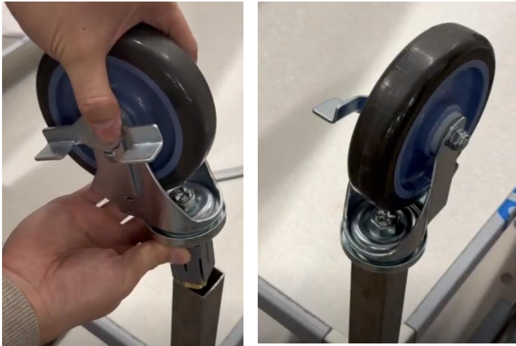
Figure 6 Insert caster assembly into UNISTAND
