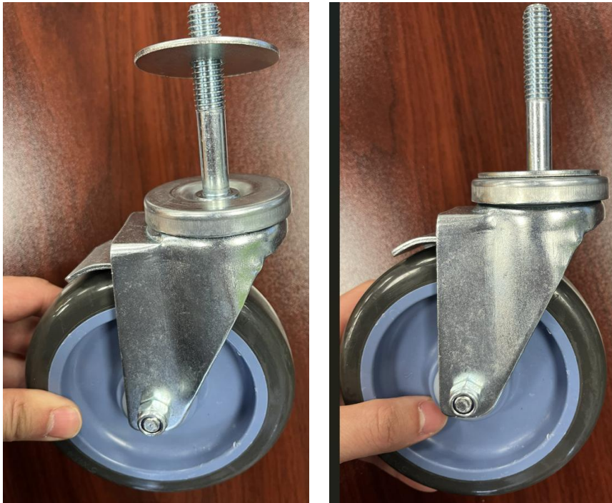
Figure 2 Place washer on caster wheel stem
