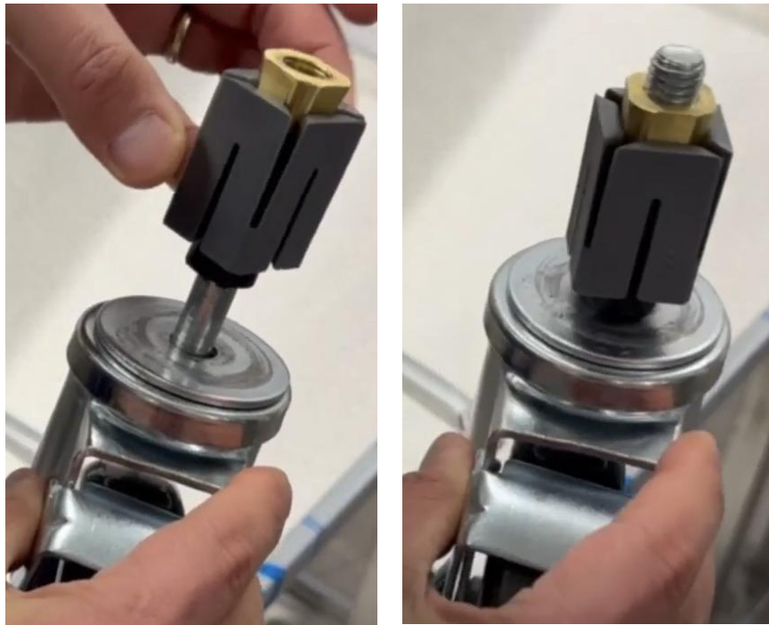
Figure 5 Hand-thread expander assembly onto caster
