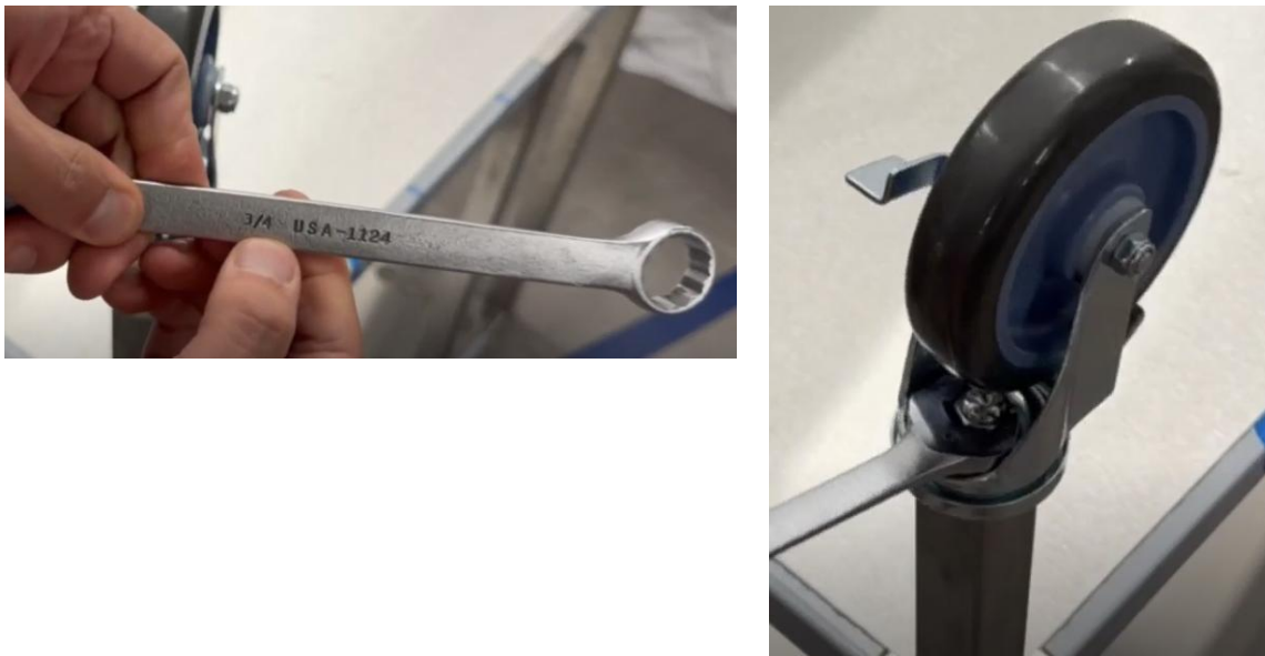
Figure 7 Tighten nut on caster assembly
