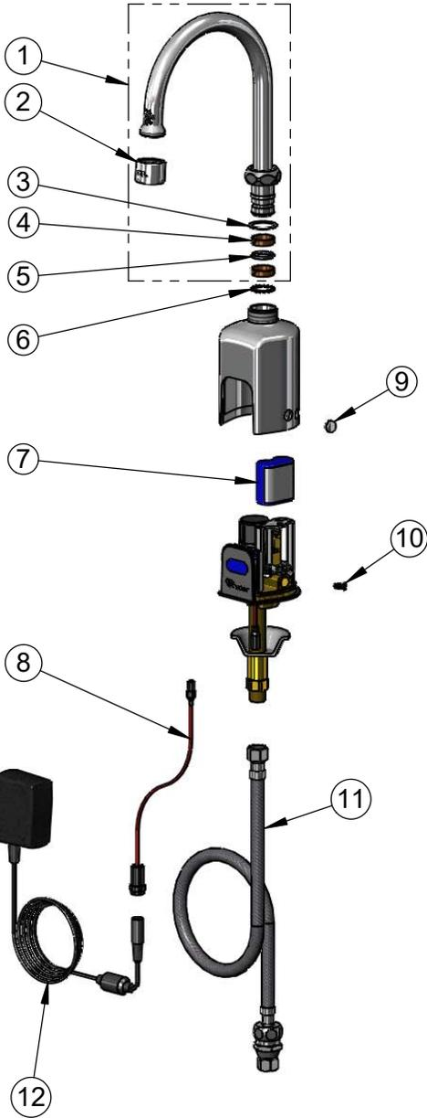
A maximum of (8) ChekPoint faucets can be powered by EC-HARDWIRE ChekPoint Hardwire AC Transformer when connected using EC-ADEWIRE cables. (Both sold separately)
