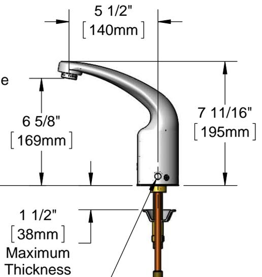
Shown w/ Optional Plug Installed When Water Temperature is Preset (Included)
