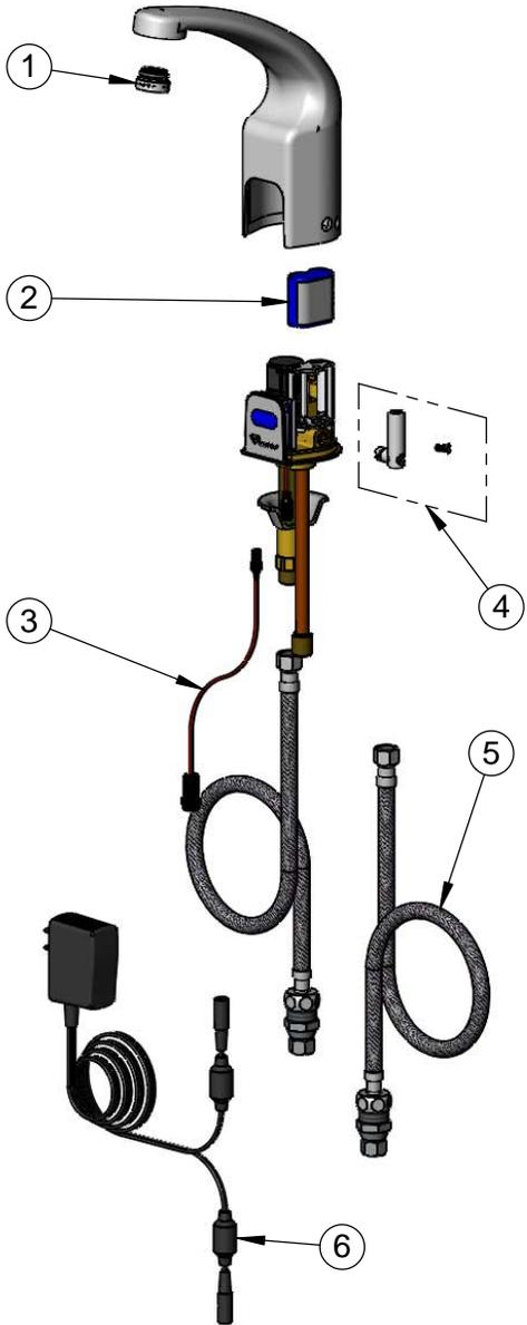
A maximum of (8) ChekPoint faucets can be powered by EC-HARDWIRE ChekPoint Hardwire AC Transformer when connected using EC-ADEWIRE cables. (Both sold separately)
