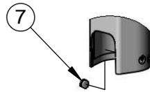
Optional Plug Replaces Lever Handle When Pre-setting Temperature (Installs from Inside of Body)
