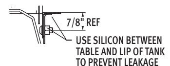
Sectional View Showing Table Connections
