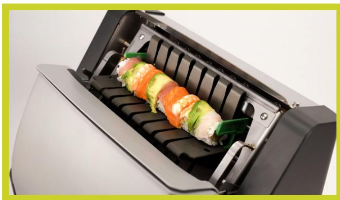
**Multiple Roll Cutting:** Because of the downward cutting action and larger cut base, up to four hosomaki can be cut at the same time.
