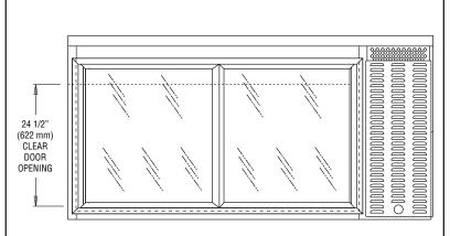
**IMPORTANT NOTE:** Models are completely front breathing and take in and exhaust air through the front grill. For proper operation, the area in front and back of the cabinet **must** not be obstructed in any way. A clearance of 3" on the sides is recommended.
