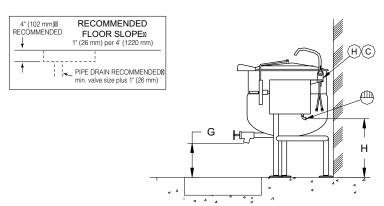
UNIT SHOWN WITH OPTIONAL 2" TANGENT DRAW-OFF VALVE, SPRING ASSIST COVER, HOT AND COLD WATER FAUCED AND STEAM CONTROL KIT.
