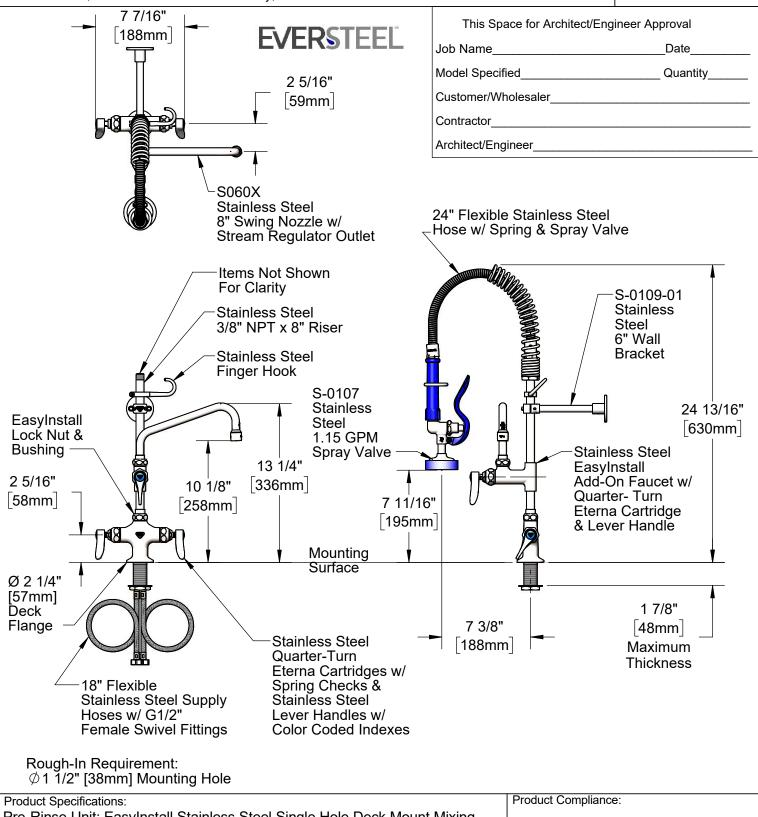
Pre-Rinse Unit: EasyInstall Stainless Steel Single Hole Deck Mount Mixing Faucet, SS Quarter-Turn Eterna Cartridges w/ Spring Checks, SS Lever Handles, SS Add-On Faucet, SS 8" Swing Nozzle, 24" Flexible Stainless Steel Hose, SS 1.15 GPM Spray Valve, SS 6" Wall Bracket & Flexible Stainless Steel Supply Hoses
