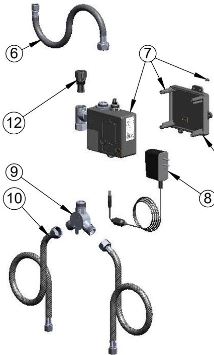
A Maximum of (8) ChekPoint Faucets can be Hardwire Connected and Powered by EC-HARDWIRE ChekPoint Hardwire AC Transformer. (Sold Separately)
