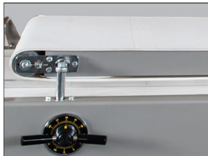
Motorized Moulding Plate with Fine Height Adjustments
