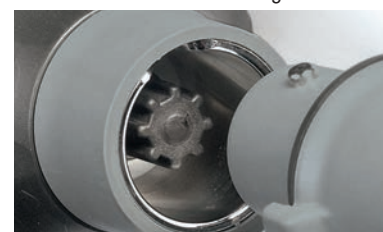
Feed tube "bayonet" slot. Changing shaft is quick & easy.
