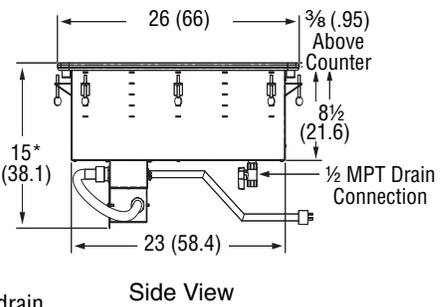
\*Manifold drain adds 6 1/2 (16.5) to overall height
