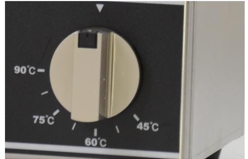
The temperature is controlled by an adjustable temperature dial which ranges from 45°-90°Celsius.
