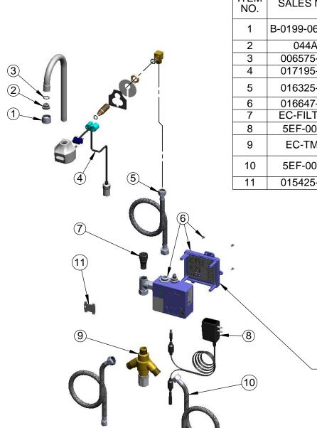
ITEM **DESCRIPTION** SALES NO. VR 0.5 GPM Non-Aerated Spray B-0199-06-N05 Device, 55/64-27 UN Female w/ Key 3/8" to Aerator Adapter 044A 006575-45 O-Ring Angled Sensor w/ Cable 017195-45 Inlet Hose, Faucet, 1/2" NPSM-F x 016325-45 3/8" NPSM-F 016647-45 **EC-FILTER** Replacement Filter 5EF-0002 A/C Transformer ASSE 1070 Thermostatic Mixing Valve **EC-TMV** Supply Hose, 9/16"-24 UN Female x 5EF-0005 1/2" NPSM Vandal Resistant Key 015425-45
