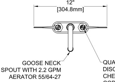
QUARTER TURN CERAMIC DISC CARTRIDGES WITH CHECK STEMS AND COLOR CODED INDEXES
