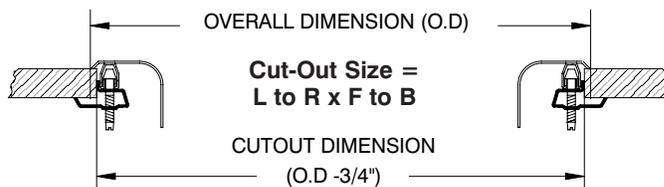
Standard Mounting Clips Fit Countertops Over 7/8" & Up To 2" Thick.
