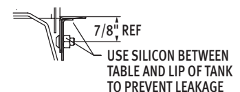
Sectional View Showing Table Connections
