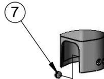
Optional Plug Replaces Lever Handle When Pre-setting Temperature (Installs from Inside of Body)
