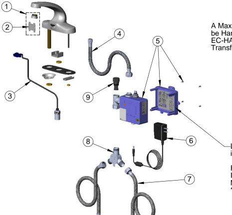
A Maximum of (8) ChekPoint Faucets can be Hardwire Connected and Powered by EC-HARDWIRE ChekPoint Hardwire AĆ Transformer. (Sold Separately)
