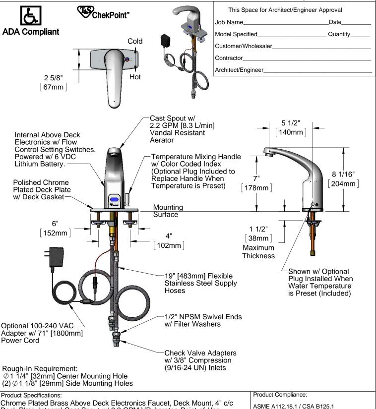
Chrome Plated Brass Above Deck Electronics Faucet, Deck Mount, 4" c/c Deck Plate, Integral Cast Spout w/ 2.2 GPM VR Aerator, Point-of-Use Temperature Control, Battery or AC Adapter Powered, 19" Stainless Steel Flexible Supply Lines & 3/8" Compression Inlets
